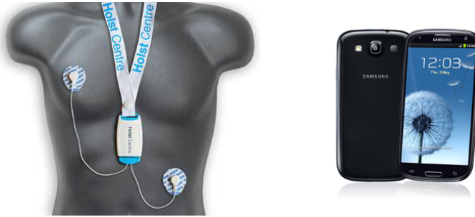
Figure 9.6: ECG Necklace and Samsung S3, the wearable sensor and phone used to collect accelerometer ECG and GPS data in this study. The ECG Necklace was worn during laboratory protocols and free living recordings close to the body's center of mass. The Samsung S3 was carried during free living only.
