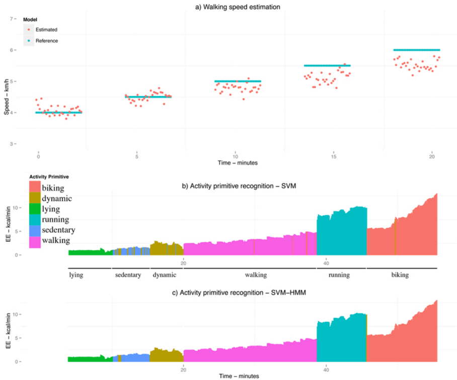
Figure 8.8: Exemplary walking speed estimation and activity primitives recognition for one participant. Activities were manually annotated and performed sequentially. Improvements in activity primitives recognition using a combined SVM-HMM compared to a single SVM are shown in plots b and c .
