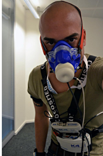
Figure 1.2: Example of indirect calorimeter, Cosmed K4b 2 .
