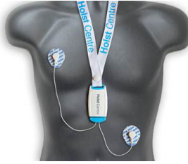
Figure 5.2: ECG Necklace. The device was used to acquire ECG and accelerometer data.
